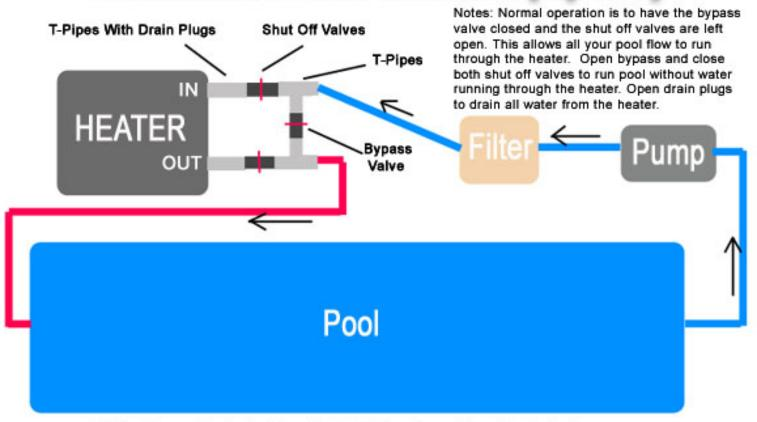
\* If you have a chlorinator, it must be installed on the red line, after the heater.
