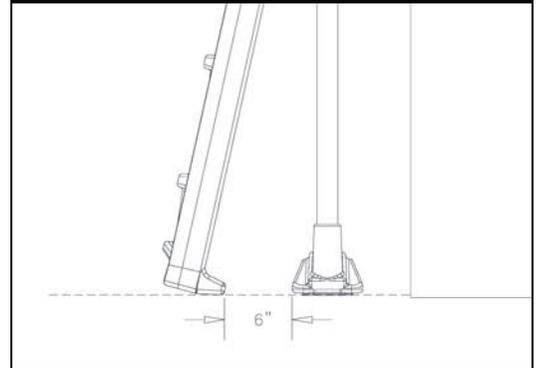
**13 -** Ensure the ladder and the base touch the ground solidly. A minimum ladder angle is required, which can be measured as a distance of 6" between the base and the foot of the ladder (fig. 12).
