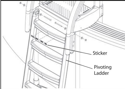
**12 -** Attach the pivoting ladder to the ramps using two 3 1/2" (2) bolts, washers and nuts. Use the top holes on the ramps for 48" high pools, the middleholes for 52" pools, and the bottom holes for 54" pools (fig. 11)
