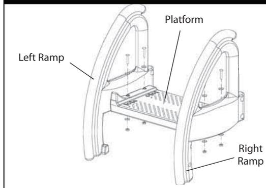
**1 -** Attach the platform to the left and right ramps using four 2" bolts, washers and nuts (fig. 1).
