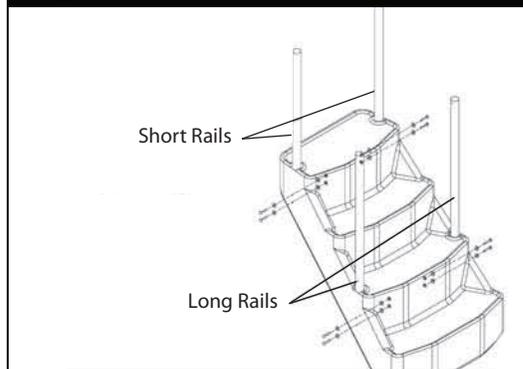
**4 -** Slide the ramps over the short rails and leave unattached. Insert the diagonal rails onto the long and short rails. From the outside of the step, attach using four 10X¾" (4) self tapping screws (fig. 4).
