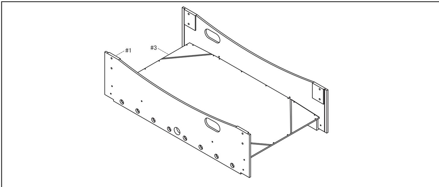
2. Attach one END PANEL #2 to each end of the table with 1/4" BOLT #10 and 1/4" FLAT WASHER #11.
