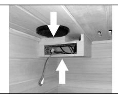
12. Plug the controller and antenna into the back of the AM/FM CD PLAYER. *Note: The red and white cables are used for an optional video player and can be tucked out of the way.* Slide and lock the AM/FM CD PLAYER into the STEREO SHELF. *Note: Use "keys" with to remove the CD player for maintenance.*
