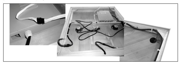
9. Feed the main power cable through hole in ROOF COVER. Secure the ROOF COVER with 3/4" SCREWS.
