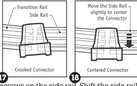
move the connector and loosen the screws on the side rail. Shift the side rail in or out from the centre of the pool until the connector can be properly centred between the rails (see diagram 18).
