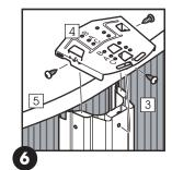
e. Line up the screw holes and fasten with one selftapping screw on each side and one on the front (key 3).
