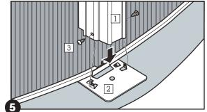
d. Hook a top plate (key 4) over the top edge of the pool wall (key 5). **Important:** Place the top plate down over the top of the vertical column with the front tab on the **outside** of the column and the side tabs on the **inside**. Make sure the vertical column is straight up and down.
