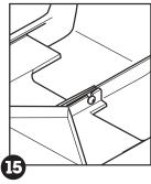
14 and 15. **Be sure** to slide the parts together **tightly**.
