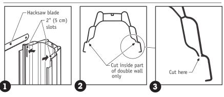
to create a slot in the double wall. Do this on both sides of the vertical. **Be sure** to cut through only the **inside** part of the double wall, and not the outside part.
