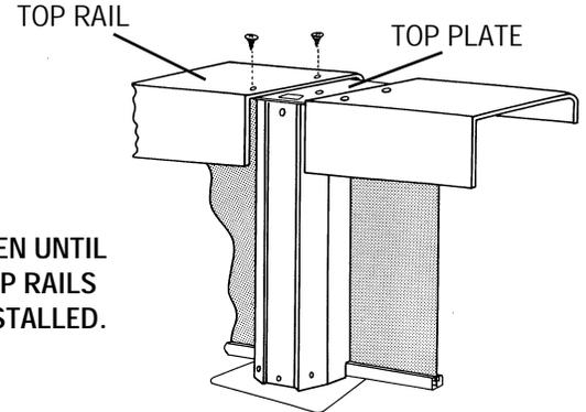
**DO NOT TIGHTEN UNTIL ALL OF THE TOP RAILS HAVE BEEN INSTALLED.**
