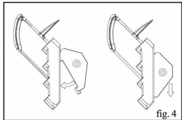
4. Slide the fence into the step and push it towards the foot of the step (Fig. 4).
