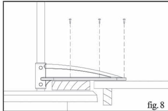
9. If the pool is lower than the deck, the braces should be shimmed\* to attain the same level as the deck (Fig. 8). Ensure the shim is properly secured to the top rail.
