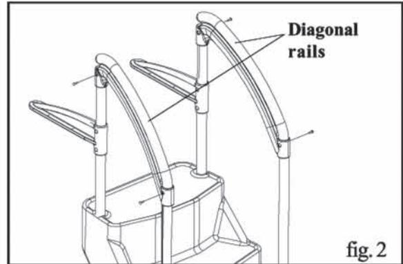
2. Insert the diagonal rails onto the long and short rails. Attach using the 10 x 3/4" screws (4) (Fig.2).
