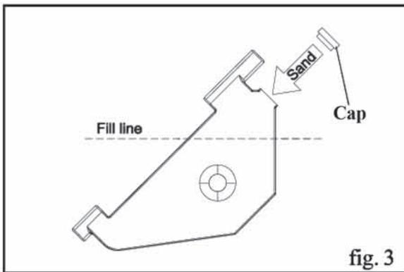
3. Pour sand\* (approx. 50 lbs.) into the fence until it is 3/4 full (Fig. 3). Install the cap properly with the 3/4" screw.
