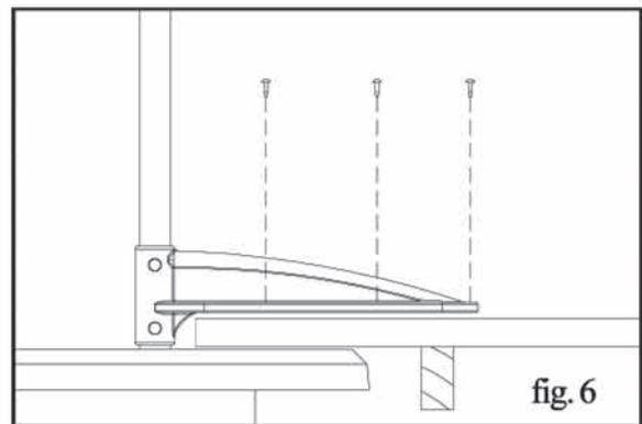
7. Attach the braces to the deck using the 1-3/4" screws (10). If the deck is above the top rail, attach the braces directly to the deck (Fig. 6).
