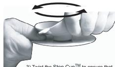
3) Twist the Step Cup<sup>TM</sup> to ensure that its mushroom has entirely cleared the wall thickness. If it has, the suction cup should rotate freely.
