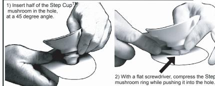
2) With a flat screwdriver, compress the Step  $\mathrm{Cup}^{\mathrm{TM}}$
