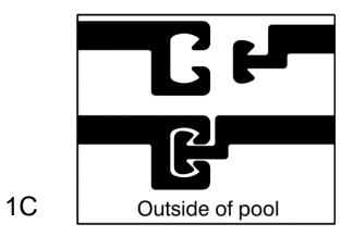
There are several different kinds of slats that go on your pool. The Beam slats have two large ribs on them. You should place one beam slat on either side of each pool upright. The beam slats can be 0-10 inches away from the upright. The upright should be roughly centered between the two beam slats. The diagram below shows the pattern of beam slats to uprights.
