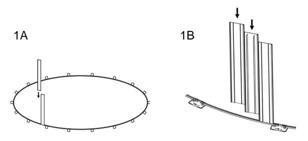
The edges of the slat should interlock as shown in diagram 1C. Make sure that the smooth surface of the slats, are facing in toward the wet side for the pool and the ribs and bumps are facing outward toward the dry side of the pool.
