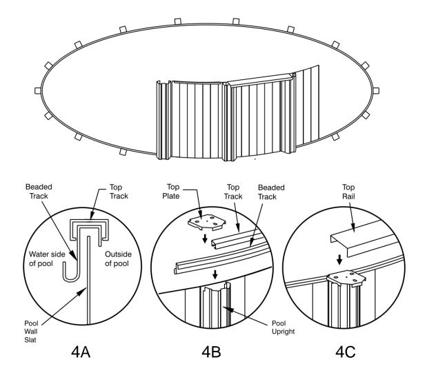
Eventually you will close up the pool wall. Sometimes the last slat can be tricky to install. You may have to open up, or close up, the bottom rails in order to get the final slat into place. Remember that we supply 10 extra slats with your pool in case you had some slats that did not install properly due to damaged or twisted ends. You should always end the installation with 10 extra slats.
