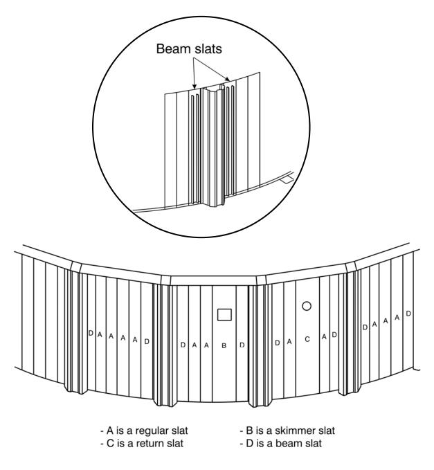
Continue to install slats until you have a section of wall about five feet long. Once you have completed a five-foot section, you are ready to start to install the pool frame onto the pool wall. See diagram below showing section of pool wall that is long enough to start to install the frame.
