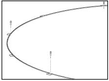
FOR 24' POOLS: Measure from bottom plate to opposite bottom plate at every other plate. When true, stake into position.
