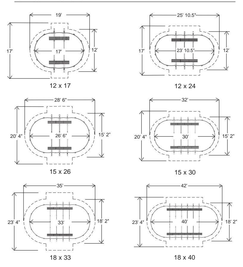
Note: All above diagrams are for Buttress-Free oval pools. If you have a traditional Buttress oval pool, you will need to add 3 feet to the width of the space needed for installation. The length measurement will not change.
