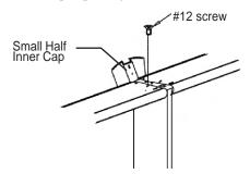
2) Attach the resin outer Top Cap using a #12 screw into hole. Put the grill over the screw when finished. See Diagram below.
