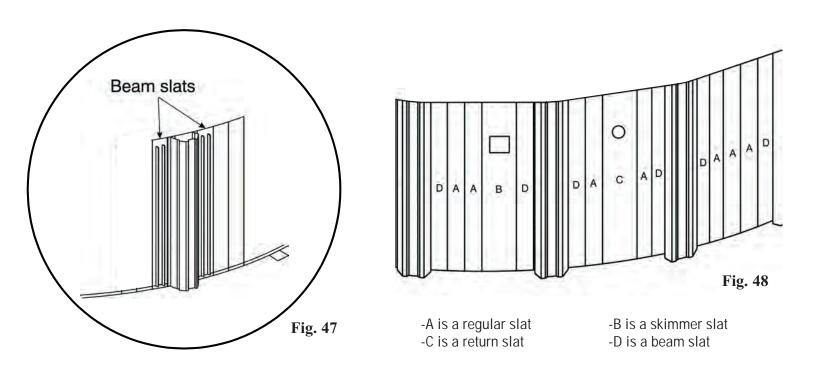
Continue to install slats until you have a section of wall about five feet long. Once you have completed a five-foot section, you are ready to start installing the pool frame upright onto the pool wall.
