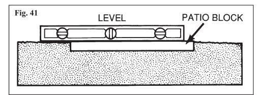
NOTE: Check for levelness in all directions. When placing patio blocks under curved side bottom plates or bottom cuffs, leave 1" of the block inside the pool and 6" showing outside of the pool.
