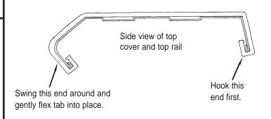
Bullnose rail is used for the illustration, but installation is the same for all 1 pc. clip-on resin covers.
