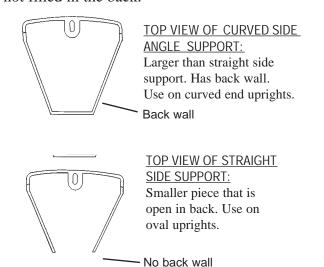
ONE PIECE RESIN CLIP-ON COVER: This installation requires no hardware. Simply hook the back end of the top cover into place, and use your fingers or a screwdriver to gently flex the front tabs enough to hook the cover in place. Make sure that the top cover is centered over the upright when installing.
