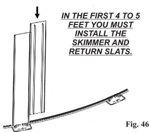
The several different kinds of slats that go on your pool are to be located in a specific order. The diagram below shows the pattern of slat types plates once your slat wall assembly is eventually completed. Frame uprights and top rails are shown at this time for general reference only. Note that beam slats are always centered around bottom plates and uprights.
