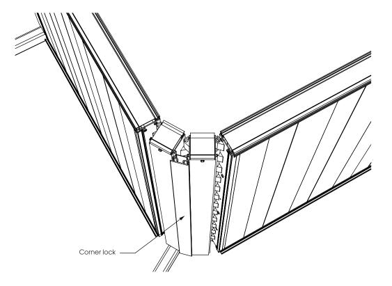
Slide the corner lock into place between the union post.
