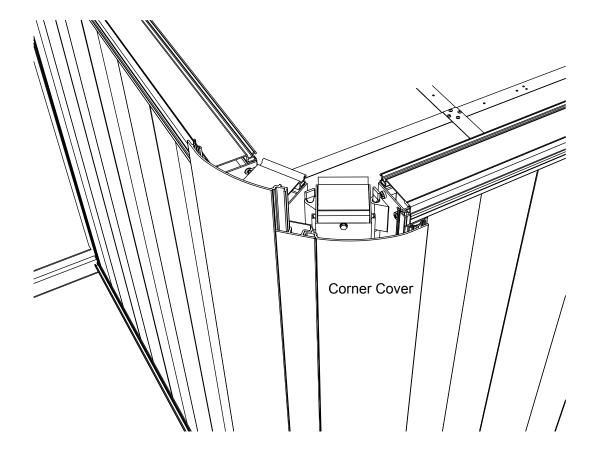
Slide the corner covers into place. They will slide into the corner lock on one edge and the receptical on the other edge.
