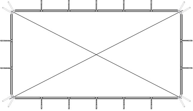
Make sure your pool is perpendicular at this point by measuring the diagonal. Both dimensions should be the same.
