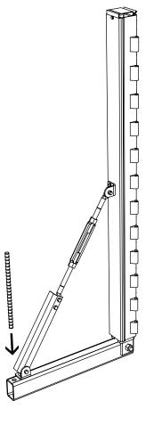
Secure the "L" assembly to the ground by inserting a rebar 1/2 (#4) x 12" long through the base rectangular tube.
