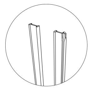
Using pliers, "crimp" the end of the radius lock to prevent the part to "drop through" when installed
