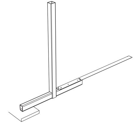
Start with the straight section of the pool by installing the universal steel strap onto the steel "T" support using 2 screw pins 1/4-20 1/2" long, with serrated nuts 1/4-20.
