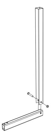
Assemble the "L" vertical post with the base rectangular tube using a screw hex 5/8-11 x 3,5" long and nut.
