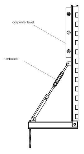
Using a carpenter level, adjust the turnbuckle in order to have the union post vertical.
