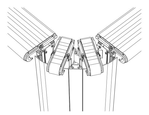
Install the small top ledges similar to the way you install them in the straight section of the pool.
