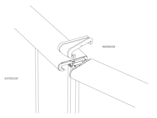
Hook the ledge cover over the ledge union, starting from outside the pool and finish inside the pool.
