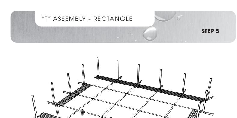
Install the pressure plate using the tapping screw # 12 x 0,75". Refer to the pool dimension pages for the correct layout according to your pool size.
