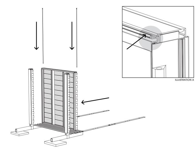
Starting in the straight section of the oval pool, insert a panel between the union posts and lock them in place using a rod on each side.
