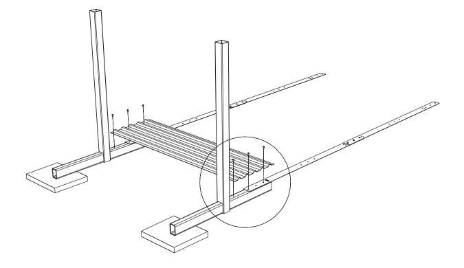
Place a pressure plate on the "T" support, but do not screw in. This will enable you to align them correctly.
