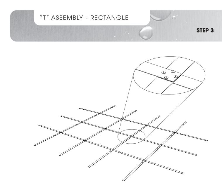
Assemble the universal straps in a criss-cross pattern using the  $1/4-20 \ge 0.75$  screws and bolts. Refer to the pool dimension pages for the correct layout according to your pool size.
