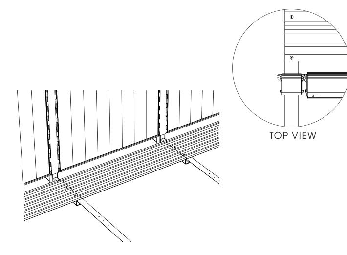
At this point you can tight up the screws holding the pressure plate to "T" support, and the screws on all universal steel straps.
