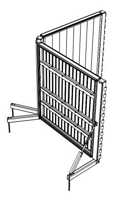
Starting in the straight section of the oval pool, insert a panel between the union posts and lock them in place using a rod on each side.
