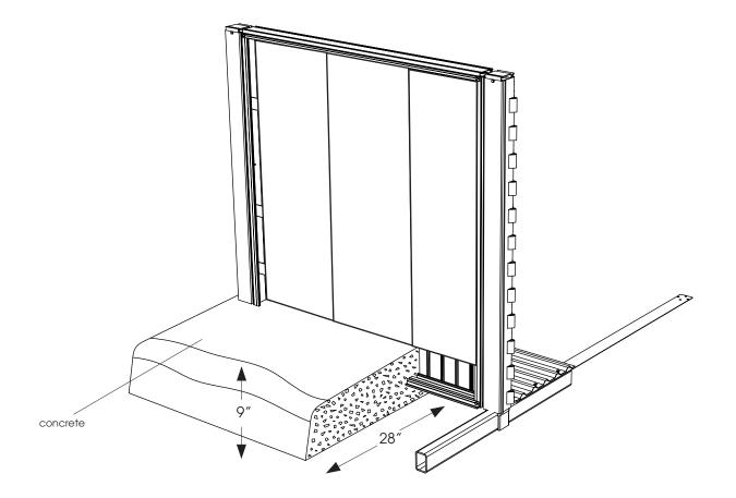
Pour a collar of concrete all around the pool at the base of the panel. Make sure the panel is level.
