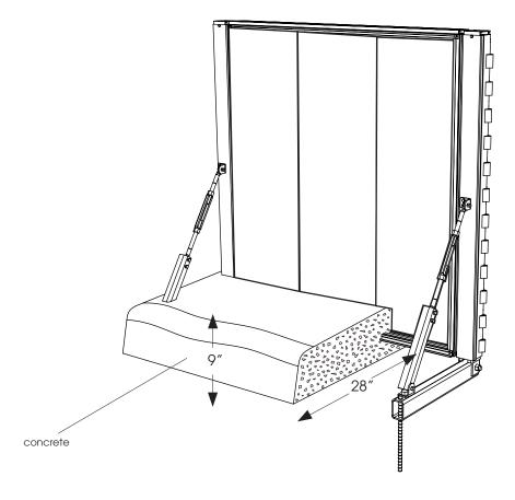
Pour concrete all around the pool at the base of the panel. Re-adjust the turnbuckle if needed in order to have the union post vertical.
