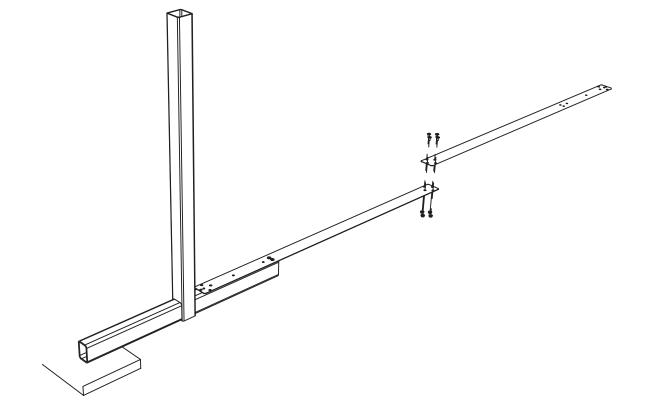
Attach all of the universal steel straps together at each joint using 4 screw pins 1/4-20 1/2" long, with serrated nuts 1/4-20.
