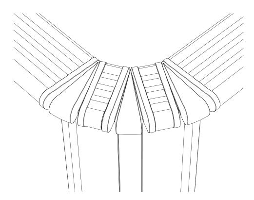
Hook the ledge cover at the corners over the ledge union, starting from outside the pool and finish inside the pool.
