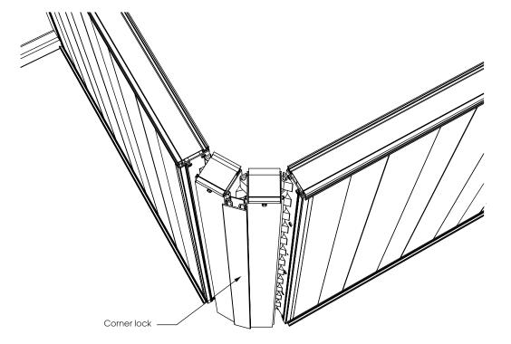
Slide the corner lock into place between the union post.
