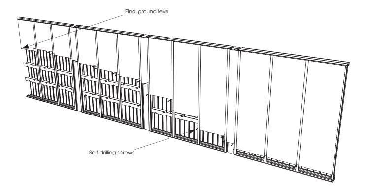
According to your installation configuration (semiinground installation), you might have to custom cut the cosmetic panels.
