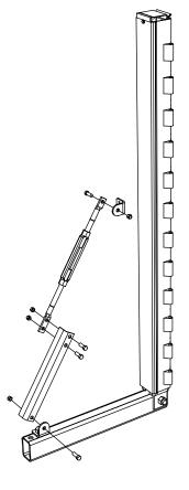
Assemble the angle turnbuckle, the turnbuckle and angle bracket to the end fitting turnbuckle using 4 screws hex 3/8-16 x 1" long and nuts.
