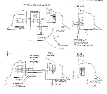
Note: Wire the pump directly to the time clock—do not use the SRS as a junction box.
