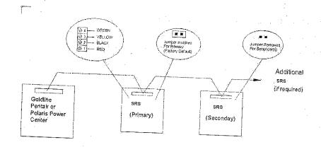
Goldline-Attach wires to proper screw terminals as show below.
