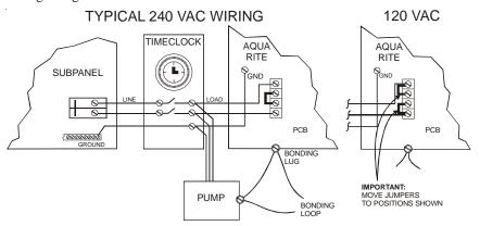
Note: Wire the pump directly to the timeclock--do not use the Agua Rite as a junction box.
