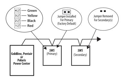
Goldline: Attach wires to proper screw terminals as show below.
