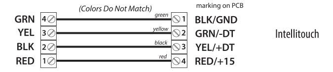
**Polaris:** Attach wires to proper screw terminals as shown below. Note that screw terminal "1" is marked on the Polaris PCB.
