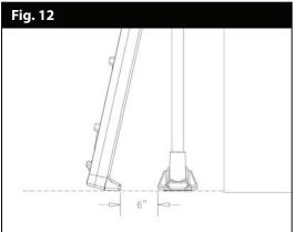
**13** - Ensure the ladder and the base touch the ground solidly. A minimum ladder angle is required, which can be mesured as a distance of 6" between the base and the foot of the ladder (fig. 12).
