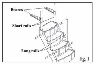
1. Insert the rails into the step (short rails on top) and align with the predrilled holes. Attach using the 3" bolts (8), washers (16), and nuts (8). Slide the braces over the short rails and leave unattached (Fig. 1).
