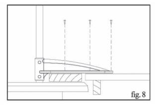
9. If the pool is lower than the deck, the braces should be shimmed\* to attain the same level as the deck (Fig. 8). Ensure the shim is properly secured to te toprail.
