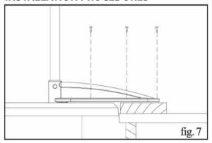
8. If the deck is lower than the pool, the braces should be shimmed\* to attain the same level as the pool (Fig. 7). Ensure the shim is properly secured to the deck.
