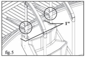
5. Lower the step into the water. Move it to its permanent location and level it horizontally.
