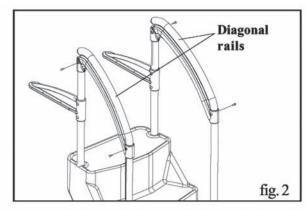
2. Insert the diagonal rails onto the long and short rails. Attach using the  $10 \times 3/4$ " screws (4) (Fig.2).
