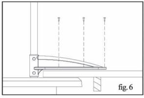
7. Attach the braces to the deck using the 1-3/4" srews (10). If the deck is above the toprail, attach the braces directly to the deck (Fig. 6).
