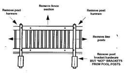
Step 3 Remove the post hardware used to secure section in place (both sides of section). Keep this hardware & remember positioning as you will require it to reassemble. Remove fence section & remove the two line posts. Keep all hardware for reassembly, Note: you may have some extra hardware left over once complete as line posts have double for opposite, sections: DO NOT REMOVE MOUNTING BRACKETS FROM POOL UPRIGHT POSTS
