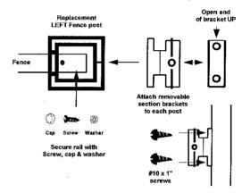
Step 4 Replace the two line posts removed with the two end posts provided. Note: there is a left and right end post included, Left & right are determined by the pre-drilled screw holes as shown above (left & right always determined when facing pool from the outside). Secure post in position using the hardware removed in Step 3 (similar to removal). Attach removable section brackets to end posts using the #10 x 1" screws provided. Repeat for all four brackets. Note: open end of bracket UP as
