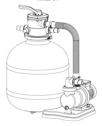
Sand not included. USE ONLY No. 20 Silica Sand with a particle size of 0.45 mm - 0.55 mm
