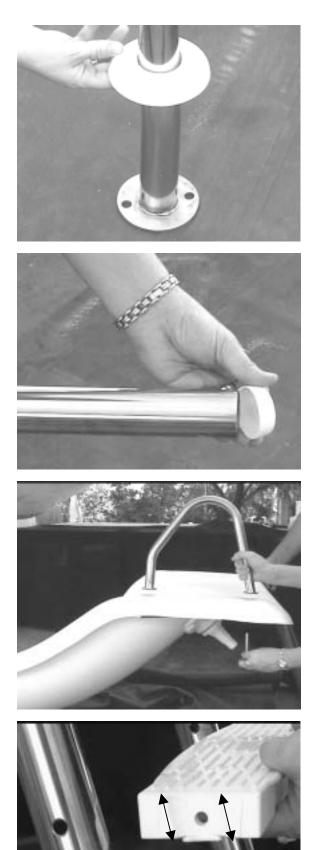
1. Slide acrylic escutcheon (looks like a doughnut – it's used to cover the ladder flange and hardware at the base of the ladder) over the open rail end. Installed correctly it will cover the flanged end of the rail.
