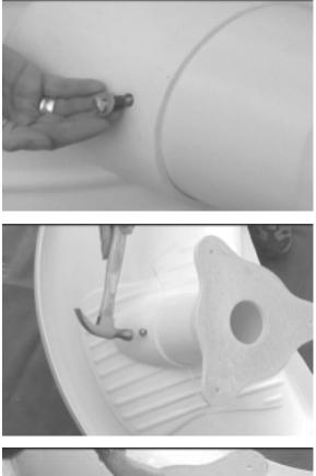
1. Align pre-drilled holes in the flume support pipe with those of the receptor on the underside of the flume.
