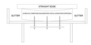
Important: nuts should be tightened slowly with 1/4 to 3/4 turns at a time. It may take a few days for the shuffleboard to completely react. DO NOT over tighten, as this can cause permanent damage to the Climatic Adjusters and your table.
