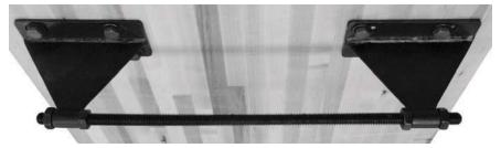
• Begin the adjustment process by placing a straight edge across the playfield directly above the first Climatic Adjuster at either end of the table. This will determine if the playfield is concave or convex. The shuffleboard surface should be slightly concave to prevent the pucks from falling off the sides of the playfield. A single sheet of paper should easily slide under the straight edge at the center of the playfield.
