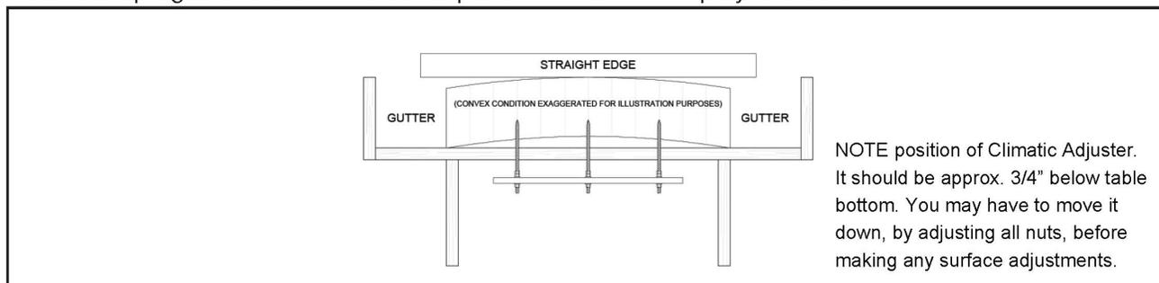
To correct a concave playfield, loosen the nut below the metal bar. Slowly tighten the nut above the metal bar down against the bar in order to push the center of the playfield up.
