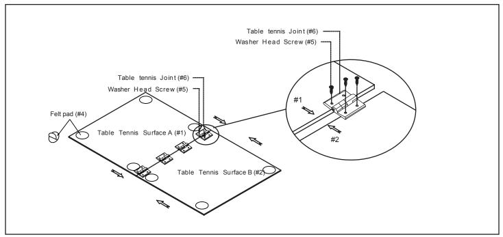
NOTE: Be sure to measure surface table is to be placed on, so felt pads #4 are positioned to contact this surface.
