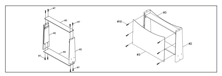
2. Attach each assembled LEG to the bottom of the TABLE BODY #1 with LARGE BOLT #15 and 5/16" FLAT WASHER #6.
