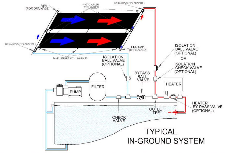
NOTE: ISOLATION VALVES ARE USED TO ENSURE WATER DOES NOT ENTER COLLECTORS DURING FREEZING CONDITIONS
