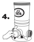
• Carefully insert control dial back into housing.
