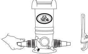
Screw adapters into each end of POOL FROG® Cycler. Hand tighten. Finish tightening by turning 1 to 2 revolutions with wrench. DO NOT OVER TIGHTEN.
