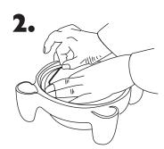
• Take hold of the far end of the o-ring with the thumb and index finger of the other hand. Roll o-ring slightly back towards you as you stretch the o-ring into the remainder of the cap groove.
