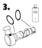
Replace both o-rings. Apply silicone lubricant that came with your POOL FROG® Cycler on o-rings.
