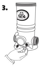
• Unscrew knob from the front of POOL FROG® Cycler. Allow all water to drain.
