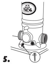
For better stability, POOL FROG® Cycler may be mounted on a base using Phillips pan head screws. One in front and two in back.
