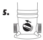
• Replace locking pin by pushing it through the slots on the dial until it locks into place.
