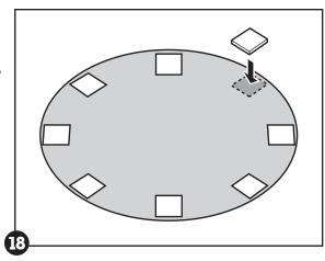
d. The patio stones **must** be sunk into the ground so the tops are flush with the soil around them. Use the carpenter's level to make sure the patio stones are perfectly level and flush with the ground. Use the carpenter's level and a 2-by-4 between patio stones to make sure the stones are level with each other.
