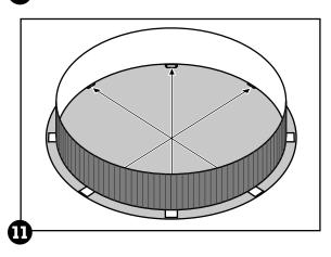
b. Adjusting the pool to the proper shape may cause the base rails and base plates to slip out of alignment a little. Recheck all of the base plates to make sure each one is centred where the base rails meet.
