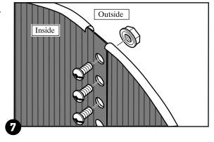
e. Cover the seam and bolt heads on the inside of the pool wall completely with 2" (50 mm) duct tape.
