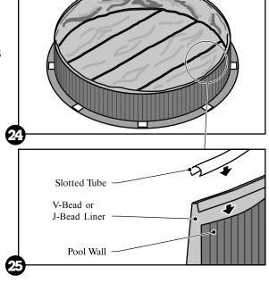
f. Start filling the pool with water. As the pool fills, work out all the wrinkles and smooth the liner to the wall.
