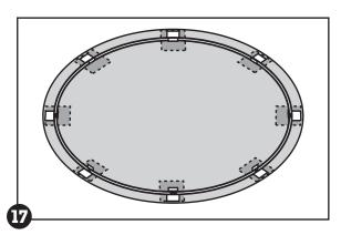
c. Remove the base rails and base plates and lay out the patio stones around the circle where the base plates were.
