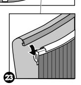
a. Remove the slotted tubes and connectors from the top edge of the pool wall.
