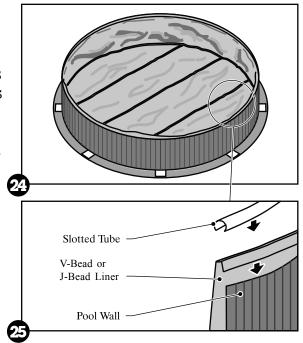
f. Start filling the pool with water. As the pool fills, work out all the wrinkles and smooth the liner to the wall.
