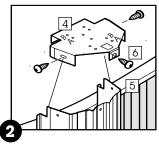
Use the ridges in the pool wall to make sure the vertical column is straight up and down.
